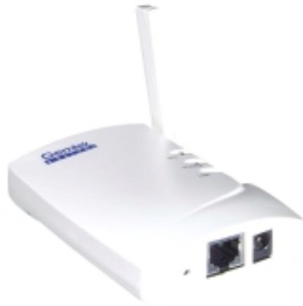
Figure 1.1 - T316 Wi-Fi Ethernet Client
