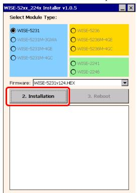
• When the process is finished, click the "3. Reboot" button to reboot WISE-52xx/WISE-224x controller.
