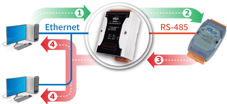
▲ In M0 mode, multiple computers can connect to the same serial device(s) via the network.
