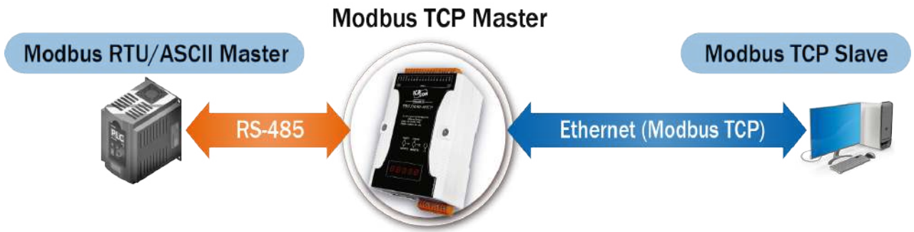
▲ A serial master can access a Modbus TCP slave device via PDS using M7/M8.
