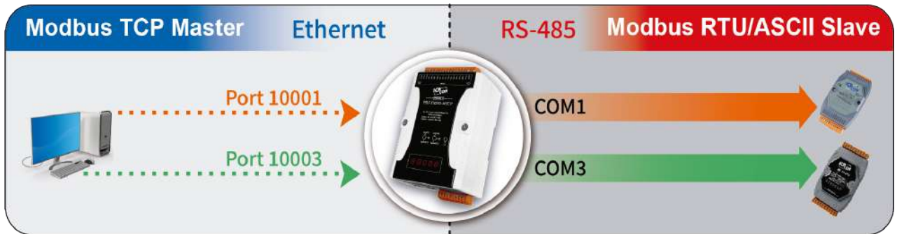
▲ In M4 and M5 modes, each COM port corresponds to an independent TCP port.
