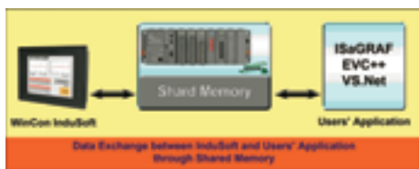
圖四：Data Exchange between InduSoft and Users' Application through Shared Memory
