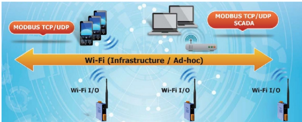
Figure 1-1 Application architecture for the WF-2000 series
