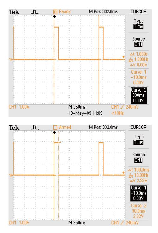
The GPS-721U-MRTU and the GPS-721U-MRTU-UTA can also be used as a time reference for radio clocks, but requires an accurate 1PPS output to be reliably used for time signals
