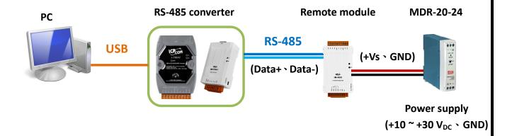
Step 2: Make sure the USB driver is correctly installed if use USB to RS-485 converter.
