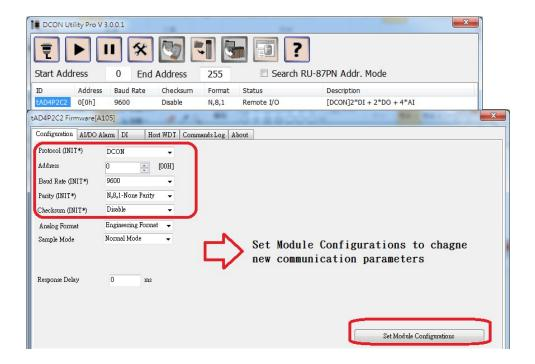
For most case, user can find the module by using steps as above, if still failed to found, the most is caused by the RS-485 bias issue, follow next section to verify and solve the problem.
