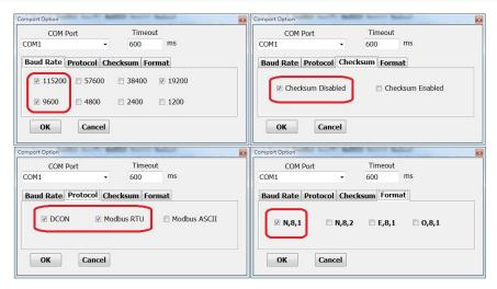
Step 4: Search the module and change the new communication parameters
