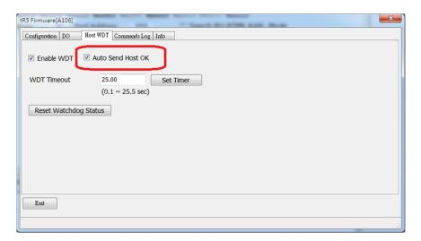
DCON must send ~ \*\* broadcast command to reset WDT Timer, Modbus module resets WDT Timer when it detects a command from the network
