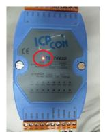
If the main program is still communicating with the module, the red power indicator will be flashing at high speed, which is easy to be mistaken for constant on. At this time, you can disconnect the communication line or close the control program to see that the power indicator will flash once every 1 second.
