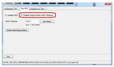
Modbus module can set whether to allow output after host watchdog timer timeout.
