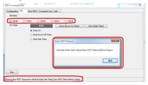
Owing to not know how to use the Host Watchdog and Safe Value, or accidentally start the Host Watchdog Timer, which causes the field personnel can't understand why the system cannot output correctly.
