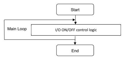
If communication is lost during heating process, the output module can not receive any commands from host PC to turn off the heater, it is very dangerous under this condition. In other words, it is unreliable in practice, and there are safety concerns.
