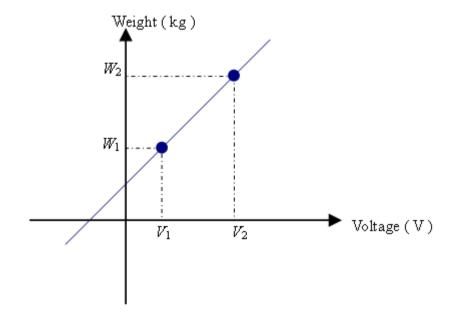
$$Gain = \frac{W_2 - W_1}{V_2 - V_1} \qquad Offset = W_1 - Gain \times V$$
