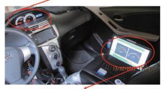
Monitor the CAN data of the engine and vehicle Speed via the I-7565-H2.
