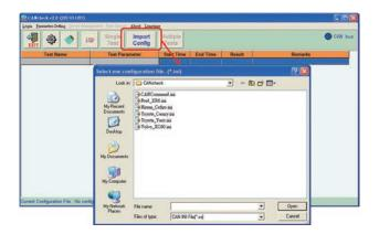
Different CAN message sets can be stored in different configuration files. The user can easily pipe different configuration files for different test cases. For example, a car factory can store several different cars' data in different configuration files, and then call the corresponding one as needed to test each car.
