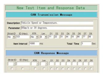
Users can model the vehicle CAN protocol or other special CAN protocol, set to the CANcheck software, the software will be able to follow the CAN command set and command transfer cycle. Users could provide the meaningful description for each CAN command. This helps to manage and identify all the complex CAN commands.
