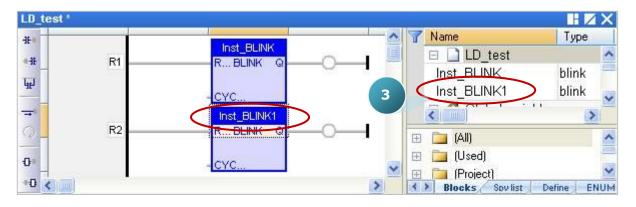
6. Click the "Coil" on the right of the "BLINK" function block, and continuously click the "Insert Coil" button to add four "Coil".
