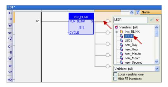
8. As the screenshot below, mouse drag-and-drop the "Output1", "Output2" and "Output3" variables to the 3th, 4th and 5th "Coil".
