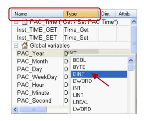
**Note:** For the function block can work correctly, the "Inst\_xxx.." FB instance variable will be automatically added when using one function block. For the safety reasons, this FB instance variable will not be automatically deleted even if the function block has been removed in the editor area. So, users can right-click the unwanted variable and select "Clear" to manually remove it.
