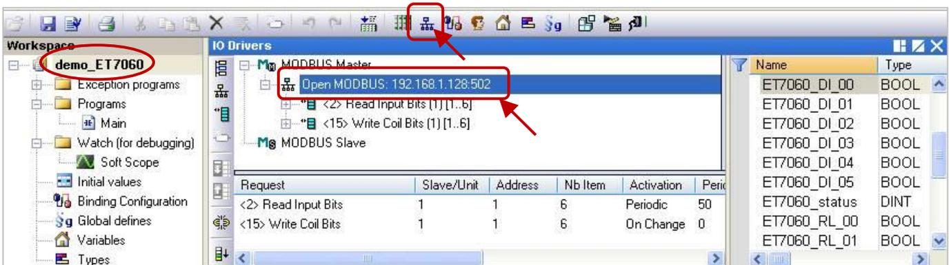
2. Double click "Open Modbus: IP:502" to open the "MODBUS Master Port" window.
