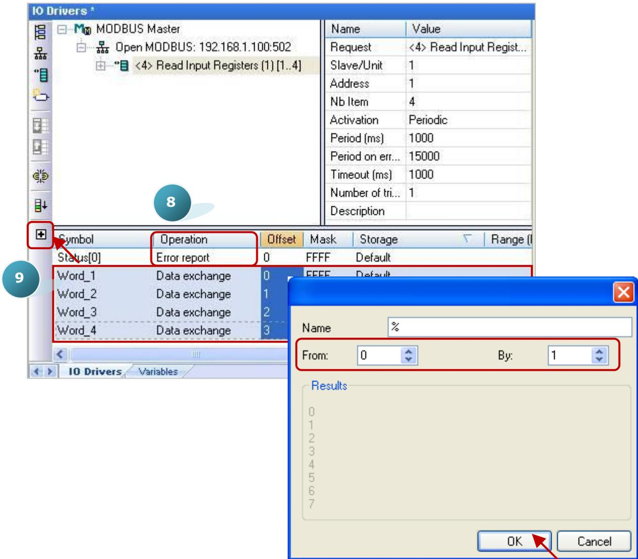
Now, we have finished the setting to read AI data. In the following section, we will describe how to read/write the DI, DO, and AI data of the ET-7000 module. You can also refer the FAQ-009 to know the configure way to read/write the DI, DO, AI and AO data.
