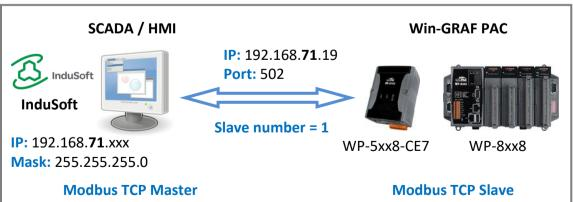
After completing all the steps, the HMI/SCADA software can access to all the Win-GRAF variables listed above via Modbus TCP protocol.
