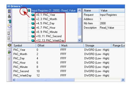
10. Then, we need to add the second "Data Block" for the Modbus Master to read the Boolean data. This configure way is similar to the step 4 to 8:
