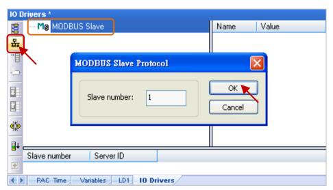
4. Click the "Insert Slave/Data Block" button on the left side to open the "MODBUS Slave Request" window.
