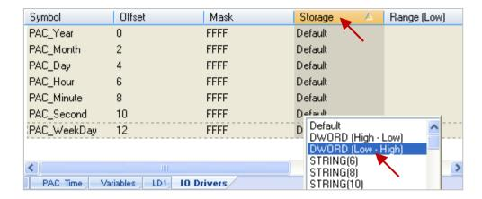
To expand this "Data Block" and you can see the Modbus addresses of all variables. It equals to the "Offset" value plus "1" (Base address).
