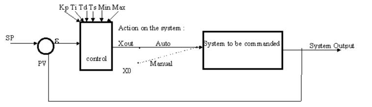
PV is the output. At the entry the error e is calculated as the difference SP-PV. The control calculates the action to do on the system to keep the regulation.
