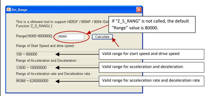
The expressions of I-8094F/I-8092F/I-8094 motion modules to calculate the speed and rate are listed below. Please refer to the module manual for detail information.
