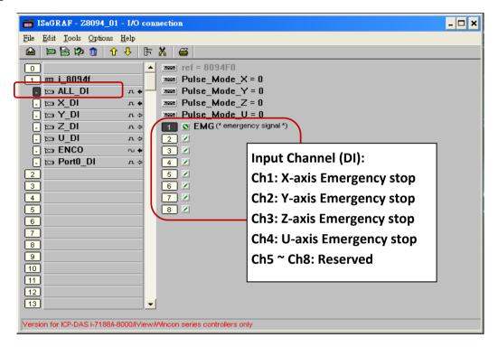
Pulse\_Mode\_X: Set the X-axis pulse output mode
