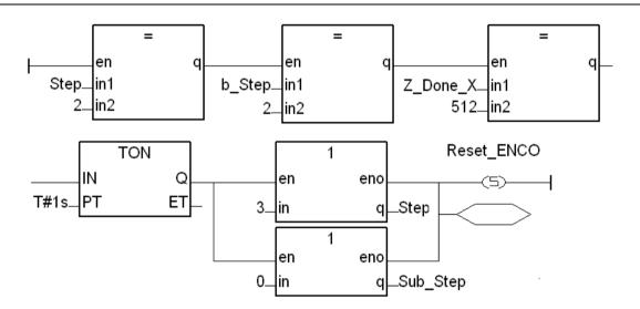
If "Step=2" and "Sub\_Step=2", use Z\_done() to check if return to the Home position. If Z\_Done\_X=512, it means Home is found, then reset "logic pulse" & "encoder pulse" to "0".
