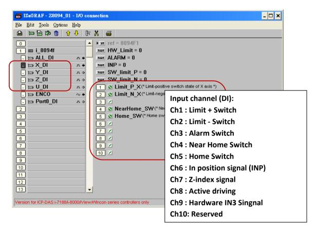
**HW\_Limit:** Setting the hardware limit positions (Limit+ and Limit-).
