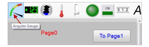
Place the Angular Gauge component in the desired position on the screen and drag the handles to resize it to a suitable size. Select the "AO Tag" option from the "Tag Type" drop-down menu, select "Word\_4" from the "Tag Name" options, and set the "MouseControl" option to "False", meaning that data can only be read.
