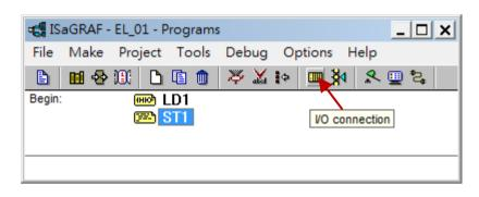
In the I/O Connection dialog box, double-click the field for "Slot 0" to open the "Select board/ Equipment" dialog box. Click the "Equipment" option in the "Library" section and then choose the "xw304" item from the list of equipment. Click the OK button to confirm your selection. The XW304 expansion board and its respective I/O channels list in the I/O Connection dialog box.
