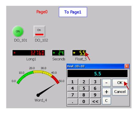
2. Verify that the value of the "Float\_5" variable in the ISaGRAF application has changed to "5.5".
