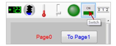
Place the Switch component in the desired position on the screen and drag the handles to resize it to a suitable size. Select the "DO Tag" option from the "Tag Type" drop-down menu, and select "DO\_102" from the "Tag Name" options. Ensure that the "ConfirmWindow" option is set to "True" which specifies that tag data can be output after user confirmation.
