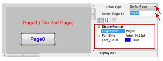
We now need to add Label and SwitchPage Button components to PageO. To do this, first expand the "Page" label in the navigation pane and click the "PageO" item to display the page. Next, follow the same process described above to add a Label component and a SwitchPage Button component to Page1, and then adjust the attribute settings so that they are the same as those illustrated in the figure below.
