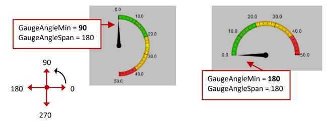
You can specify the color that different sections of the range will be displayed in, e.g., green, yellow and red, which allows you to quickly check the status. In this example, we will set the
