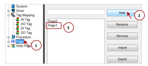
Expand the "Page" label in the navigation pane and click the "Page 1" item to display the new page. Select the desired VGA resolution for the ISaGRAF PAC from the Layout Size drop-down menu to set all pages as the same resolution.
