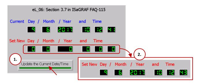
To adjust the date and time, click each component and enter a new value for the item. For example, in the diagram below, click the second's component in the "Set New" section to open the "Value Entry" dialog box. Enter the new value and click the "OK" button to save the new value. Repeat this process each item that needs to adjust, and then click the "Set as New Date/Time" button and click the "OK" button to change the information displayed in the "Current" date and time section above.
