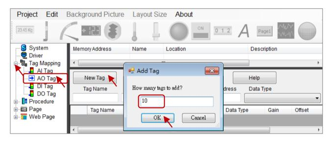
You can simultaneously edit the details of multiple tags by first selecting the first data row then holding the Shift key and clicking the last row to select all of the rows. You are then able to assign any of the data types (e.g., 32-bit Float) to all of the tags at the same time.
