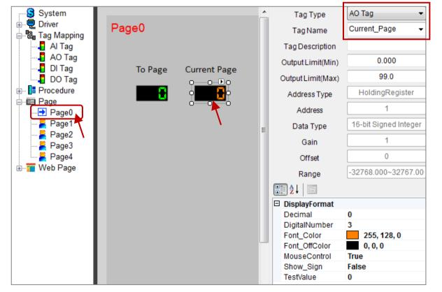
Finally, upload the ISaGRAF and eLogger projects to the PAC. See Section 1.7 and 2.6. To test that the project is functioning correctly, double-click the component ("To\_Page") to set a value on the HMI screen to verify that the HMI page switched to the specified page, and to verify that the current page number is in the "Current\_Page" variable.
