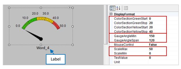
Next, set the "GaugeAngleMin" value to 150, which signifies that the minimum value is located at 150 degrees in the anti-clockwise direction, where zero is the baseline of the Angular Gauge component. Set the "GaugeAngleSpan" value to 120, which signifies that the range that the pointer can travel is 120 degrees. For example,
