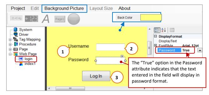
The Login web page contains two label components, two textbox components, and a button component. To configure an individual component, click the component to display the related attribute window and then modify the properties where necessary.
