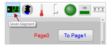
Place the 7-segment numerical component in the desired position on the screen and drag the handles to resize it to a suitable size. Select the "AO Tag" option from the "Tag Type" drop-down menu, and select "Long\_1" from the "Tag Name" options.
