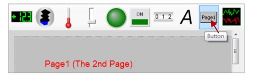
Place the Button component in the desired position on the screen and drag the handles to resize it to a suitable size. Select the "SwitchPage" option from the "Button Type" drop-down menu, and select "PageO" from the "Switch Page to" drop-down menu. Configure the desired attributes for the component in the property window, such as the display text, the font size, and the color, as illustrated in the diagram below.
