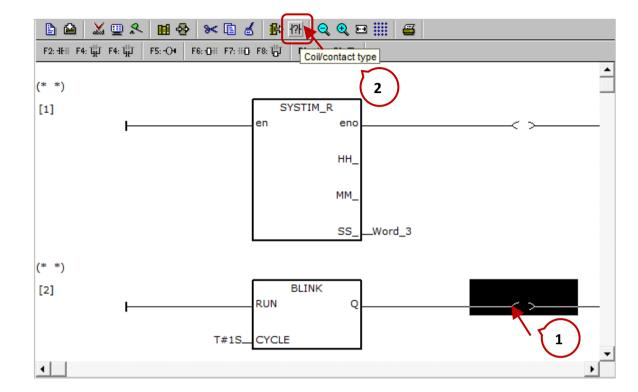
Double-click the "N" coil icon to open the Select Variable dialog box. First, select the "Boolean" option and click the "M1" option to assign the variable. Click the OK button to save the new variable.
