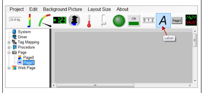
Place the Label component in the desired position on the screen and drag the handles to resize it to a suitable size. The attributes for the component, such as the display text, the font size, and the color, can configure in the property window, as illustrated in the diagram below.
