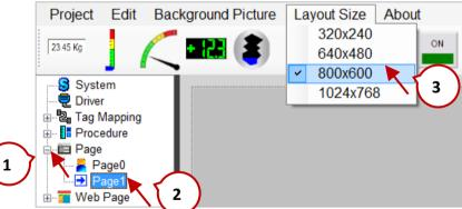
The following is an overview of the maximum VGA resolution that can select for the various ISaGRAF PAC models:
