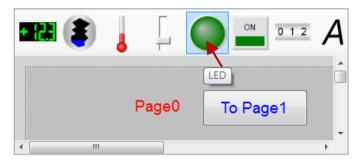
Place the LED component in the desired position on the screen and drag the handles to resize it to a suitable size. Select the "DO Tag" option from the "Tag Type" drop-down menu, and select "DO\_101" from the "Tag Name" options. In the "Display Format" section of the property window. Ensure that the "ConfirmWindow" option is set to "True", which specifies that tag data can be output after user confirmation.
