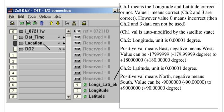
The "DO2" is two Boolean output channels in I-87211W modules.
