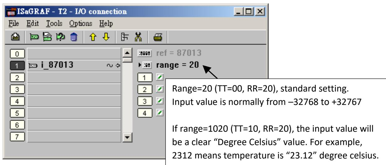
If setting range as 20 (or 21 to 2F), then it is “standard setting”. The temperature input value is 2’s compliment value from –32768 to +32767 depends on the “range” value. For example, setting range as 20, value of –32767 means temperature is about –100 Degree, +32766 is about +100 Degree. Value of 16383 means +50 Degree. (**Note:** Normally value of –32768 or +32767 means wire “broken-line”)
