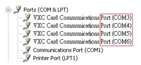
This problem usually occurs because COM1 and COM2 are set to be used by the operating system itself, meaning that you will not be able to use either of these COM Ports unless the current functions are stopped beforehand. To resolve this issue, follow the process described below to complete configuration.
