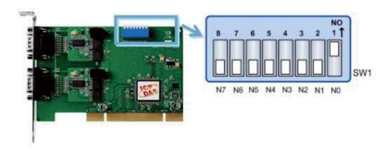
**Step 4:** Reinstall the multi-port serial card device into the computer then restart it. Once the system reboots, open the Device Manager following the procedure described above, and verify that the drivers are installed correctly. If the card is correctly installed, the COM Ports will already be set to start from COM1.
