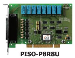
Universal PCI, 8-ch Isolated DI and 8 Relay Output Board
