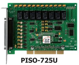
Universal PCI, 8-ch Relay Output and 8-ch Isolated DI Board
