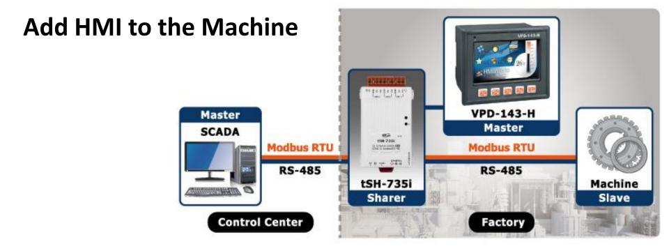
The original architecture is a remote SCADA (Supervisory Control and Data Acquisition) system connected to the machine at the factory via RS-485 for monitoring and setting. With the introduction of tSH-735i and VPD-143-H, the original remote SCADA system can still work with the machines, and the field personnel can also check and adjust the parameters of the machines in the factory to improve the efficiency of the field work.
