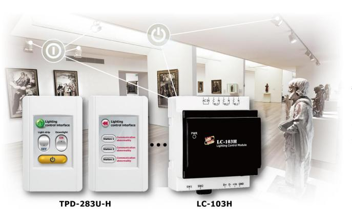
The ICP DAS LC-103H Lighting Control Module has 3 relay outputs (16A @ 250VAC, 16A @ 30VDC), each relay can control a group of lighting circuits. In addition to RS-485 remote control, it can also be connected to the local switch to easily achieve the dual switching function of physical and digital.
