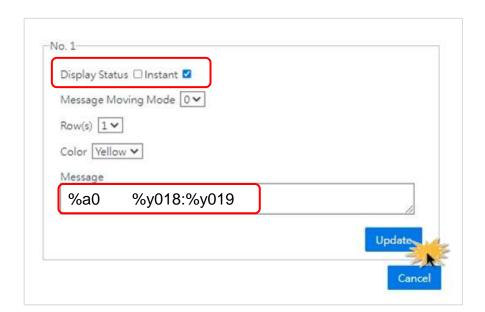
When the **Display Status** box is unchecked, the No. 1 message will not display until the box is checked manually, or the Modbus register 00100 is set to 1 to enable the display. Since an instant message has a higher priority, the display of all common messages will be suspended as soon as the display of No. 1 message is enabled.
