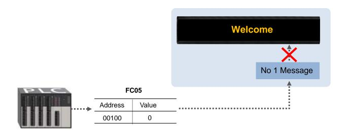
Due to the instant property of the No 1 message is checked, the display of all common messages will be suspended during the display period of No. 1 message.
