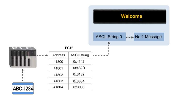
2. Send 1 to address 00100 to enable the display of No. 1 message.
