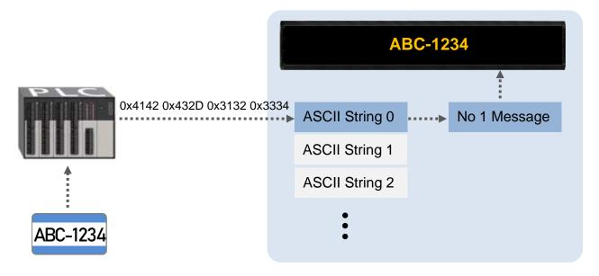
Take using No1 message to display ASCII string 0 as an example. At first, we have to get information about variable format for string 0 and time, and the Modbus addresses for the time from the user manual.
