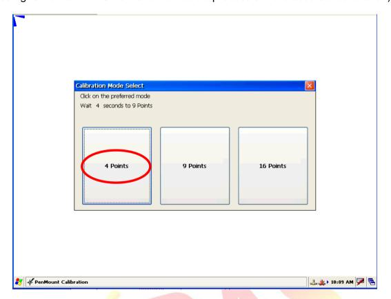
4.3. Touch the "icons on the monitor one by one to perform the calibration process.
