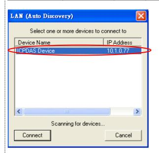
**Step 9: Double click** the searched device (such as the example above, ICPDAS Device with the IP Address 10.1.0.77), and the Windows CE desktop on the device named "ICPDAS Device" will be displayed on the Host PC.
