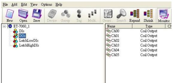
Communication will be established, and you can exchange data between XP-8000-CE6 and ET-7060.
