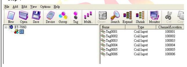
You could communicate with DI of ET-7060 now. You could also add other tags as the same way just notice the difference of address and Prototype.
