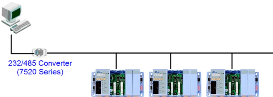
If there are repeaters on the RS-485 network, there will be pull-high/pull-low resistors on both sides of the repeaters (7510 series)
