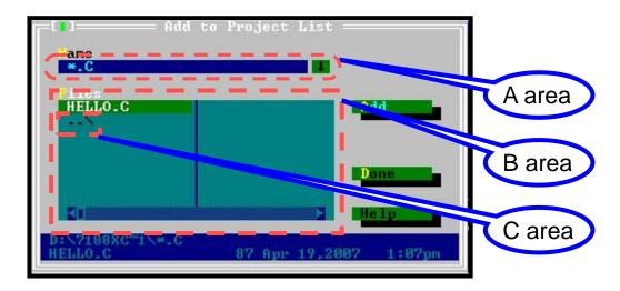
Step 7.2: Select the function library. Type "\*.lib" and press **Enter** in A area. If the file you want is in B area, moving the green block to choose the file and click the **Add** button. If not, moving the green block to C area and press **Enter** to search the file.
