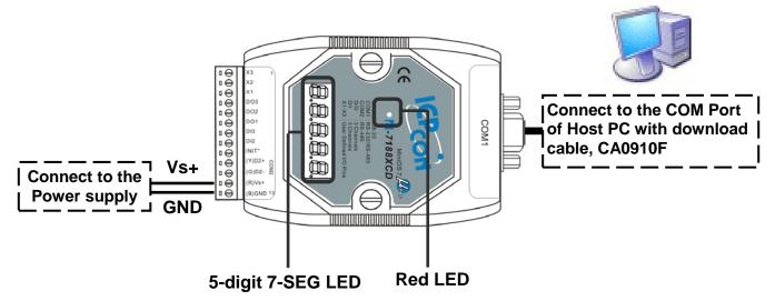
Step 3: After applying the power, the 5-digits of the 7-SEG LED will continuously show as follows.
