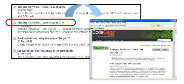
Step 3: Click on the link for **Turbo C++ version 1.01**, as shown below, to download the **tcpp101.zip** file. When requested, save the file to a safe location.
