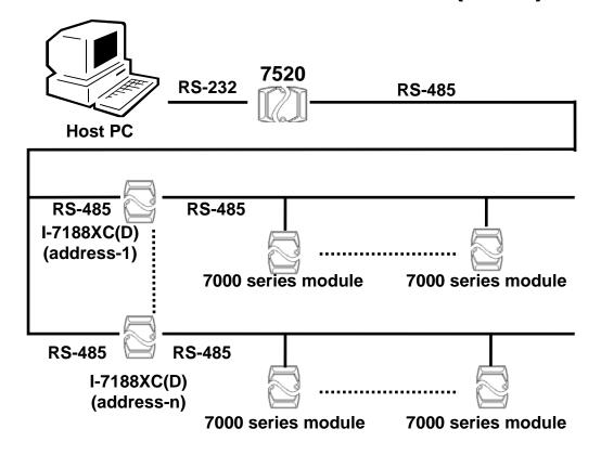
In this configuration, the 7000 series modules act as slave devices. The control programs are implemented in the Host PC. The operation steps are as follows:
