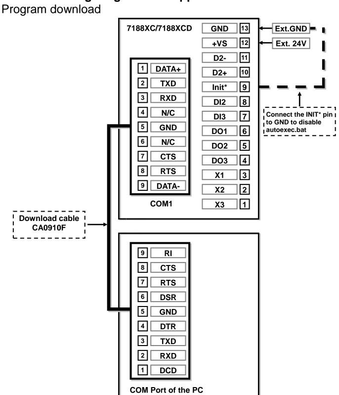
Note: Connect the DB-9 of the download cable to the COM Port of PC.
