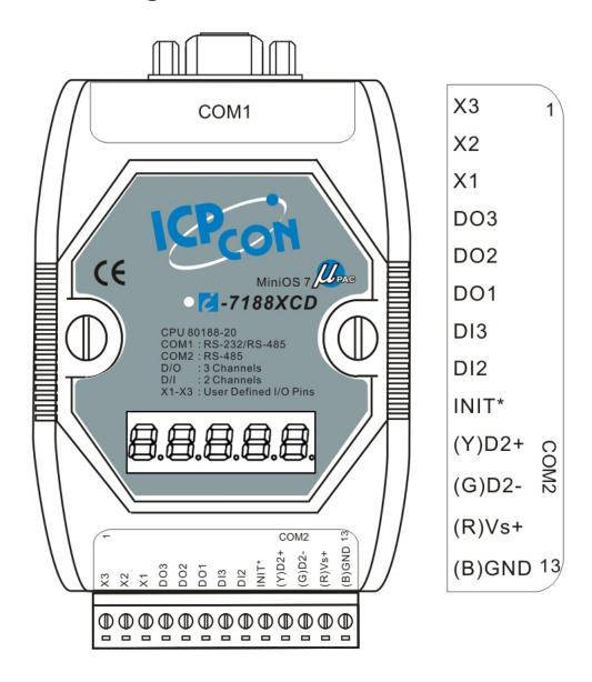
The pin assignment of 14-pin screw terminal block is as follows:
