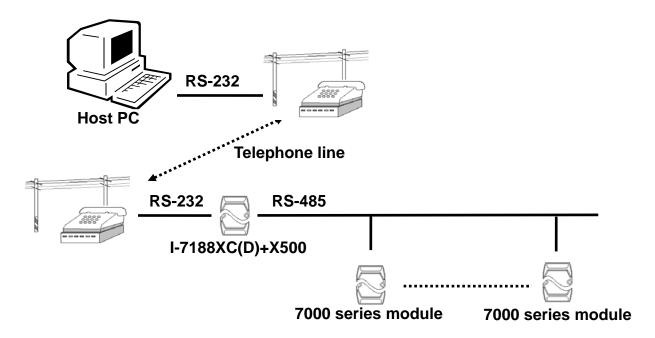
In this configuration, the control program is implemented series a local I-7188XC(D). The I-7188XC(D) will directly control the 7000 series modules based on these control arguments.
