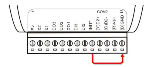
Step 2: After the I-7188XC(D) has been switched on, disconnect the INIT\* pin from the GND pin.
