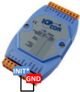
The INIT* pin connected to the GND pin
