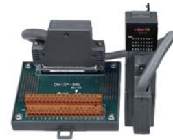
I-8041AW, I-8041W and I-8041PW with DN-37-381-A and DB37 Male to Female Cable (Optional)
