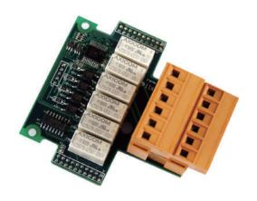
**X116**6-channel relay output and 4-channel isolated D/I
