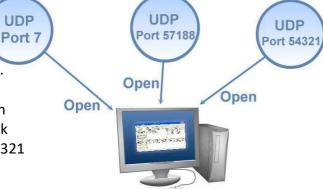
3. Utility cannot search for devices in different subnets, so confirm that the module and PC are in the same subnet.
