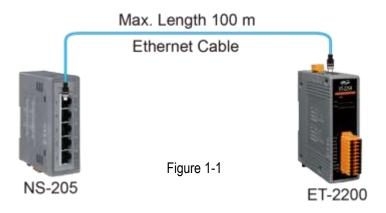
The ET-2200 series module has a built-in two-port Ethernet switch that can be used to implement daisy-chain topology. If multiple ET-2200 series modules are powered normally, then the maximum length of the Ethernet cable is also 100 meters for each upward and downward Ethernet port on the ET-2200 modules.
