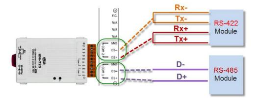
2.B: Use I-7513/I-7514U RS-485 HUB to isolate the RS-422 and RS-485 devices to avoid interference in communication.
