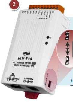
Step 2: Set the "Init Switch" to the "Init Mode" position.
