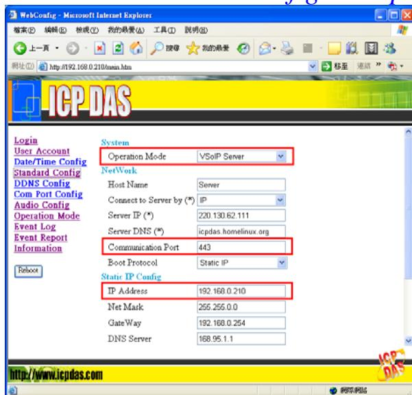
Step3: If server and client are in the local network, please confirm the network settings of client have the same domain and different IP with server.
