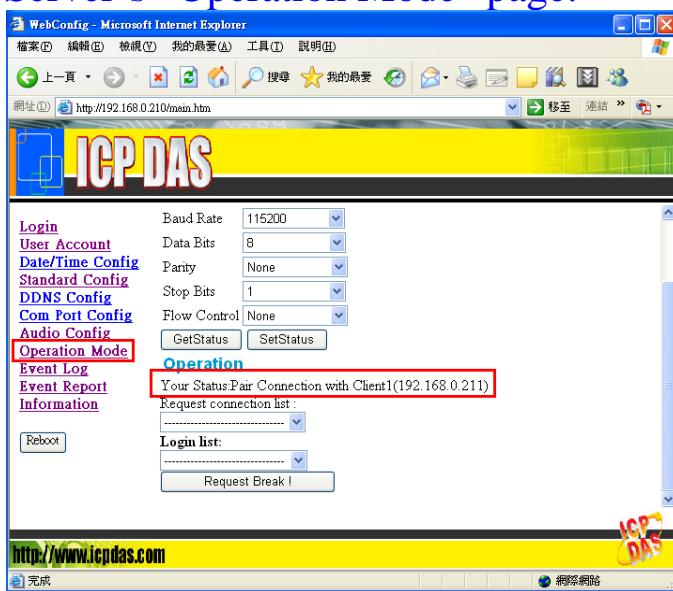
Step 3: Confirm that the Com Port device is connected with Server and Client has the same communication settings with Server's "Operation Mode" page. If it is different, please break the connection and change the settings then reconnect the client.
