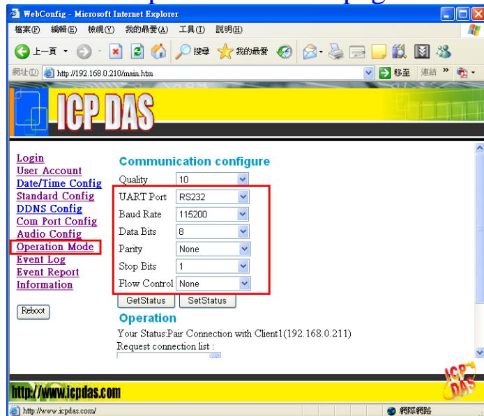
Step 4: Confirm the Cable connected Server/Client to Com Port device is wired correctly. If the connection is RS485, the user can refer to user manual section 2.2.2. If the connection is RS-232 and the Com Port device is a data circuit-terminating equipment (DCE), the user just needs to match the signal names to connect Server/Client to Com Port device, else the user needs to use a crossover cable to connect.
