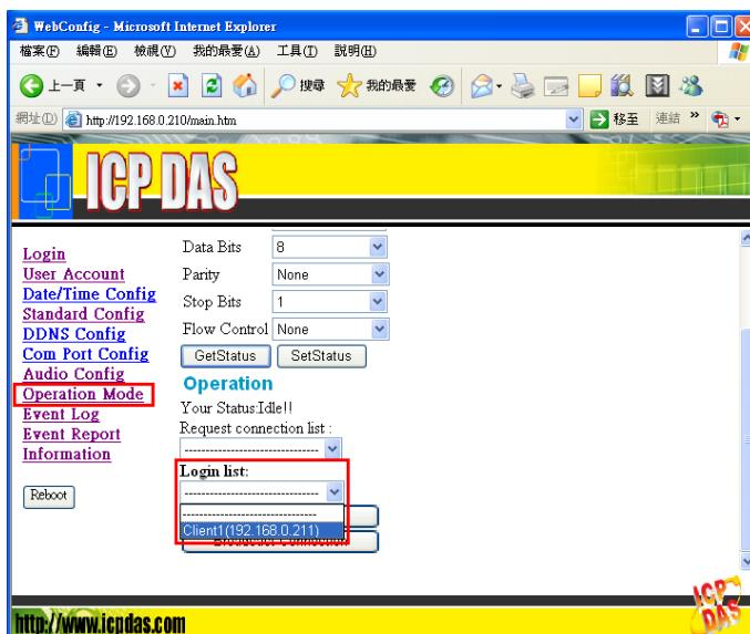
Step 2: Confirm Server and Client are at “Pair Connection” mode and it shows “Your Status: Pair Connection with Client (IP)” at Server’s “Operation Mode” page.
