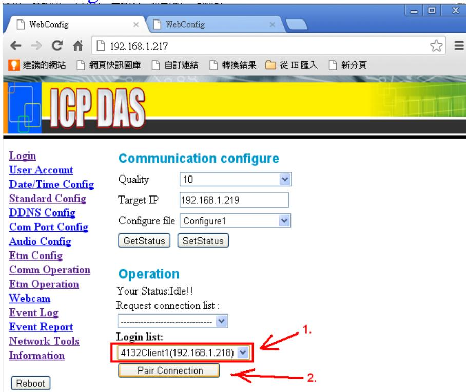
Step16: At this time, the SA2 led of server and client should flash fast. It means the Pair connection is OK. Now, the user can connect to the
