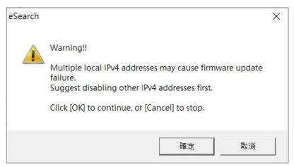
Solution: Pleaes disable the other network interfaces, leave only the single one connected to the module. RUN the update process again.
