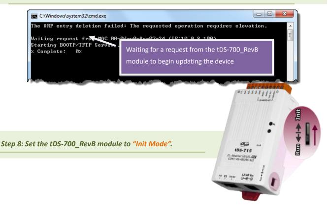
Step 9: Power-on reset the tDS-700\_RevB module in "Init Mode" to initiate the update.
