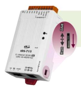
Step 11: Once the update is complete (i.e., when the progress indicator reaches 100%), set to "Run Mode".
