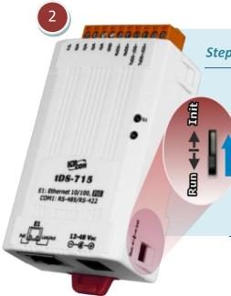
Step 2: Set the "Init Switch" to the "Init Mode" position.
