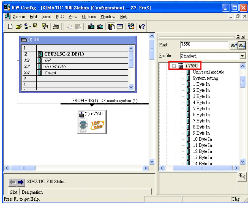
c. Click I-7550 module and double click “System setting module” and select the IO modules that you need (ex: 16 Bytes IN, 16 Bytes OUT).
