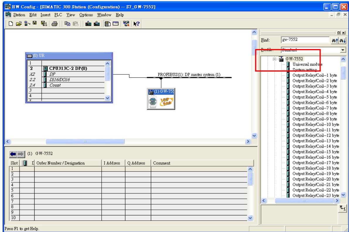
c. Click GW-7552 module and double click “System setting module” and select the IO modules that you need (ex: 2AI , 2word)
