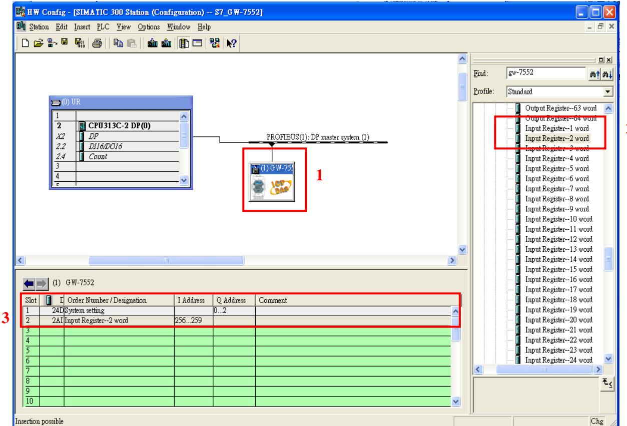
11. You have completed GW-7552's configuration and you just need to download the configuration to Siemens PLC.
