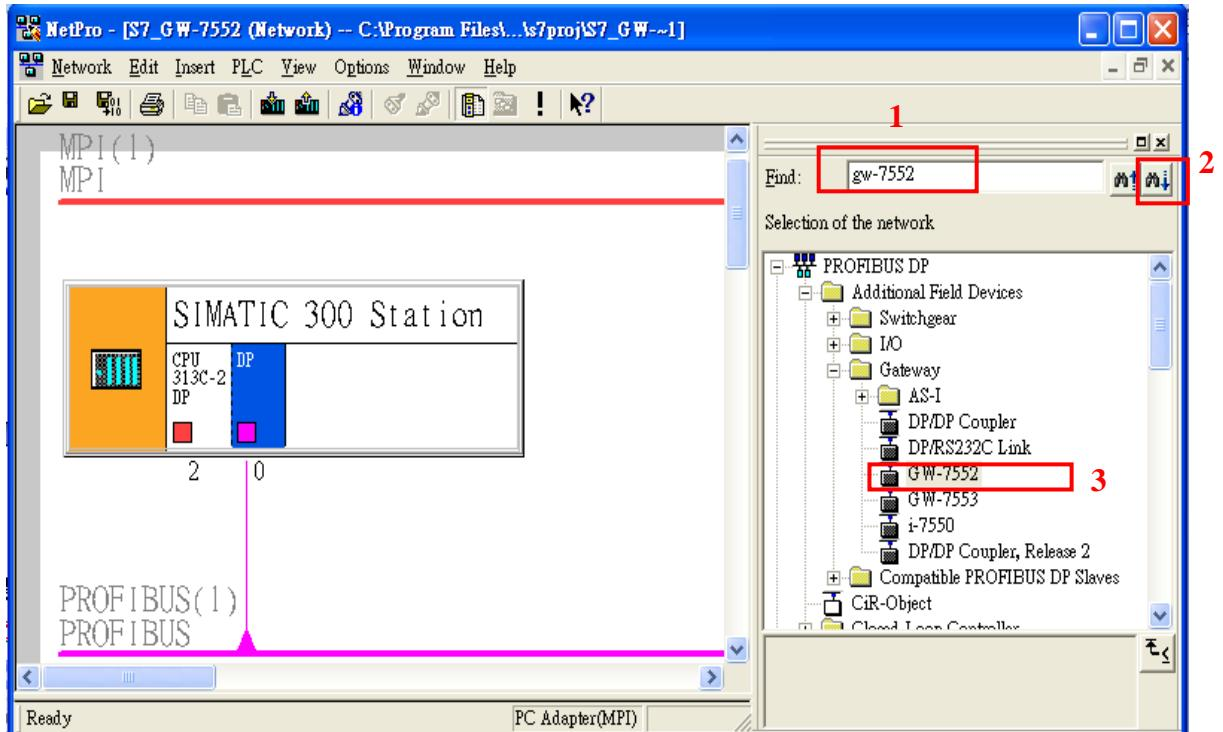
b. Select DP module and double click GW-7552's icon then set GW-7552's address in the "Properties" dialog (this address must be the same with dip switch of the GW-7552 module and default is "1") then click "OK"
