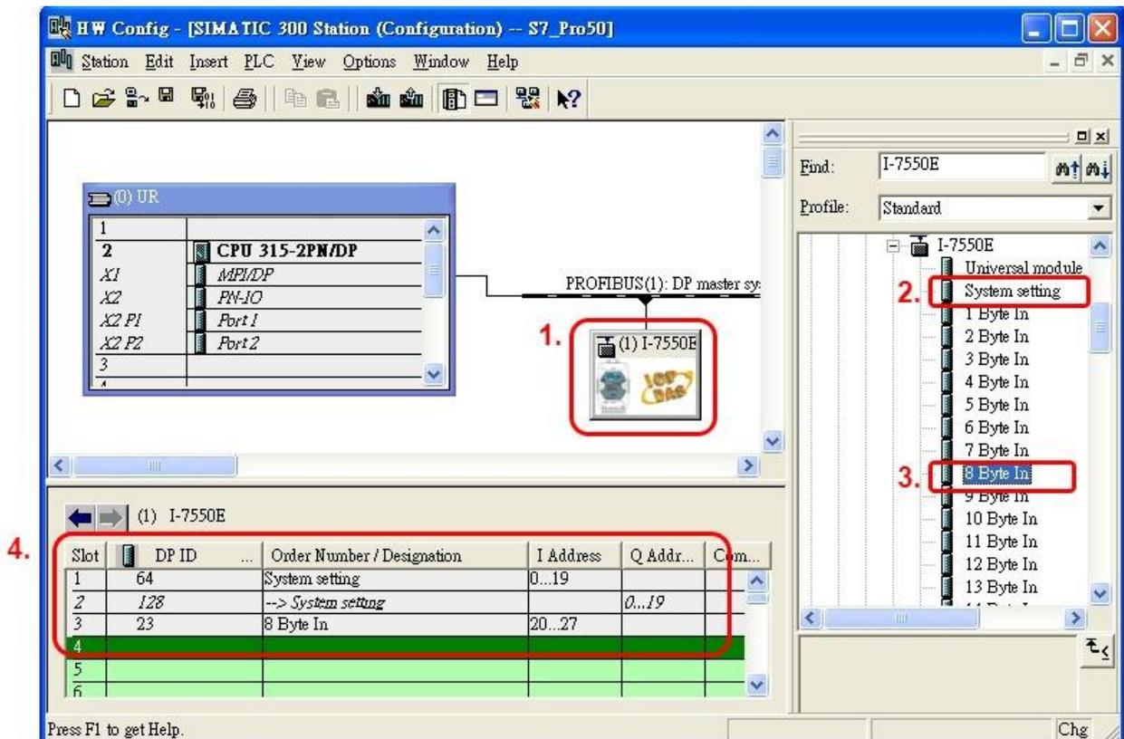
10. You have completed I-7550E's configuration and you just need to download the configuration to Siemens PLC ◦
