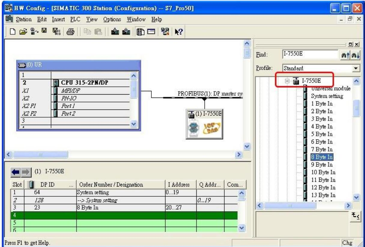
c. Click I-7550E module and double click “System setting module” and select the IO modules that you need (ex: 8 Byte In).
