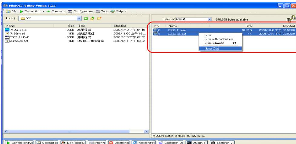
Step 10: Select the new firmware (7553vxx.exe) and autoexec.bat and upload
