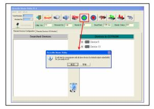
8. Clicking "Remote Device I/O Monitor" page to view the I/O data of the slave devices.
