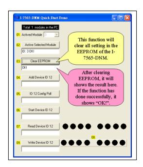
6. In this step, users can press the "Active Selected Module" button to make the I-7565-DNM to be started. The edit box below will show the result.
