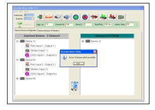
7. Pressing "Start all Device" button to communicate with all slave devices.We can ignore the warning message in this example.
