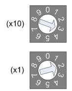
Figure 2-3 Node ID rotary switch
