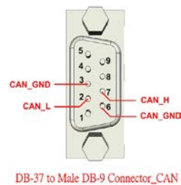
DB-37 to Male DB-9 Connector_CAN
