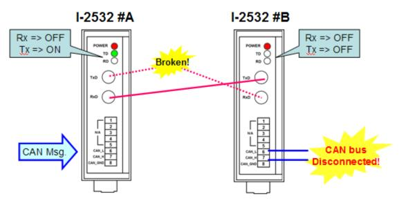
(5) Different CAN baud rate on the two I-2532 modules.
