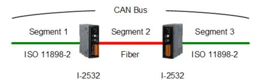
If some bus error, except the short of the CAN\_H and CAN\_L, happens in the Segment 1, the CAN error message will be transferred to the Segment 3 and vice verse. The short of the CAN\_H and CAN\_L have no affection to another Segment. That is, the CAN data exchange in the Segment 1 works normally even if the CAN\_H and CAN\_L are shorten in the Segment 3. The CAN message transformation between Segment 1 and Segment 3 is terminated while the Segment 2 is broken. (2011/1/5,Bear)
