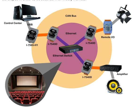
The customer in control center would like control light status and amplifier output via CAN Bus in the movie theater, but the total distance of CAN Bus between control center and CAN devices is over 1 kilometer which is beyond CAN Bus standard. In order to solve the distance issue, he uses I-7540D for translating CAN messages into Ethernet packets to control terminal CAN devices. By using Ethernet method, the CAN devices no longer have a limitation of the CAN bus distance.
