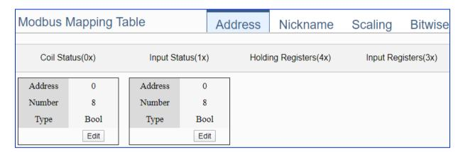
If user selects ICP DAS module, the system will auto set up the Modbus Mapping Table. If not, user needs to check the module Modbus address or I/O number from the module user manual.
