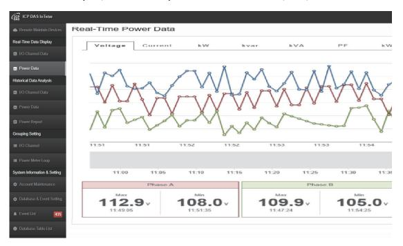
IoTstar also provides IoTstar Dashboard Service package. Through the Dashboard editor and a variety of Widget components provided by IoTstar, user can quickly setup the Dashboard page for the Real-Time sensor data (and Power data) collected from the WISE/PMC/PMD controllers according to their needs to review the operation status of the application system in real time.
