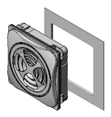
3. Rotate the front cover counterclockwise until the screw hole appears
